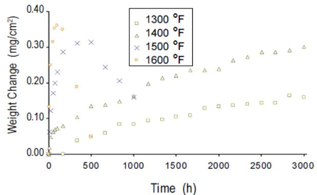
Oxidation is more complex than simple scale thickening. Spallation, or the detachment of the surface oxide scale is the most common problem encountered during the oxidation of stainless steels. Spallation is typically manifested by rapidly accelerating weight loss. A number of factors can cause spallation, chief among them are thermal cycling, mechanical damage, and excessive oxide thickness.
