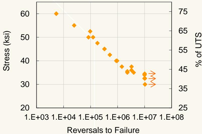
Room Temperature S/N curve (reverse bending) for ATI 334Mo® alloy
