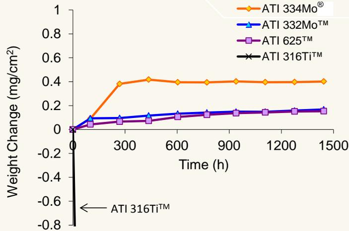
Oxidation weight change at 1400°F (760°C) in air containing 10% water vapor by volume
