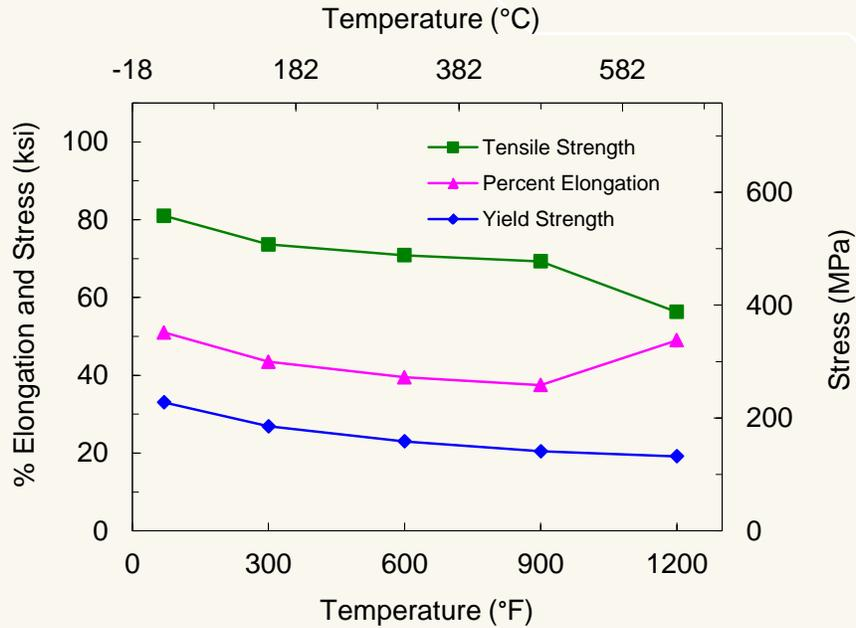
Elevated temperature tensile properties of ATI 334Mo® alloy
