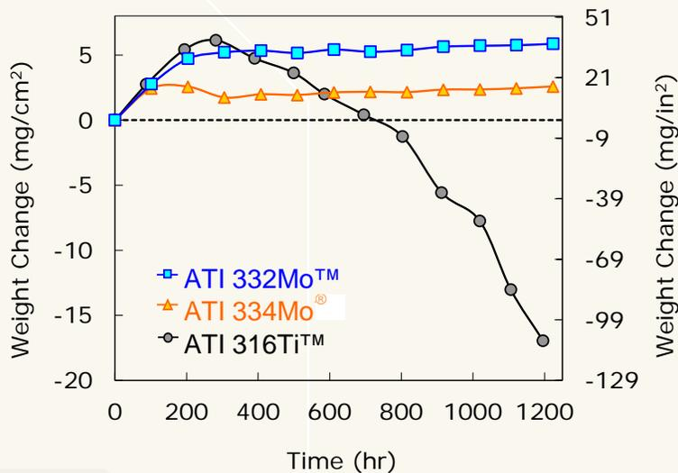
Weight change of salt-coated, welded teardrop samples exposed at 1200°F (649°C) in air under thermal cycling conditions
