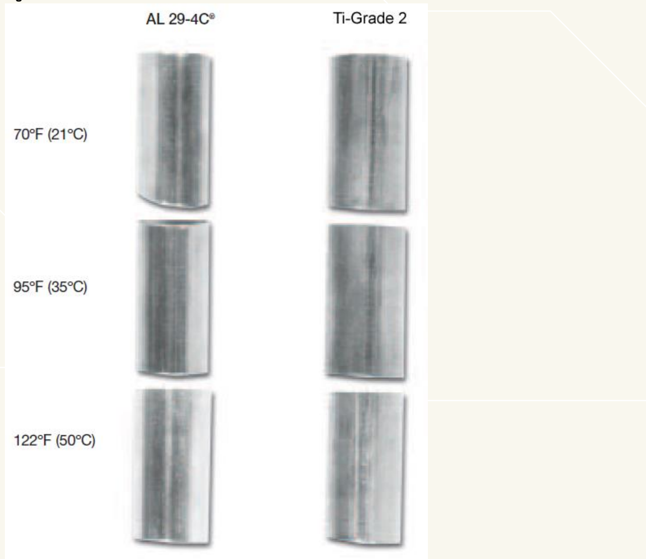
Figure 3 — Crevice Corrosion Test in Ferric Chloride for 72 Hours.
