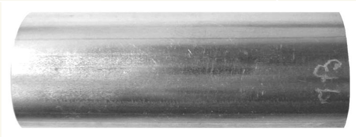
Figure 8 – Macrograph after corrosion testing of an AL 29-4C® tube that was produced properly. (Sample Length = 2 inches)
