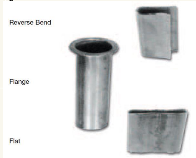
Figure 5 — AL 29-4C® Tube Tests
