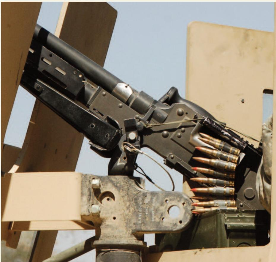
The Universal Pintal Adapter was made from ATI 425<sup>®</sup>-MIL Alloy for use with ARDEC's Objective Gunner Protection Kit (OGPK) and serves the purpose of mounting both the forward gun shield of the OGPK and standard weapons.
