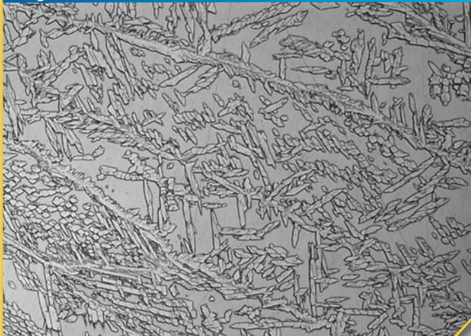
Figure 6 – Photomicrograph of a Filler Weld Fusion Zone. Finely dispersed austenite in a ferrite matrix. (200X, KOH etch)
